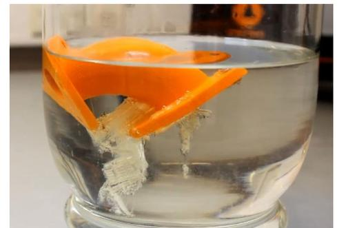
If your printer features a dual extruder, simply load a spool of ABS and a spool of PVA, and you're ready to create intricate prints with overhangs.
